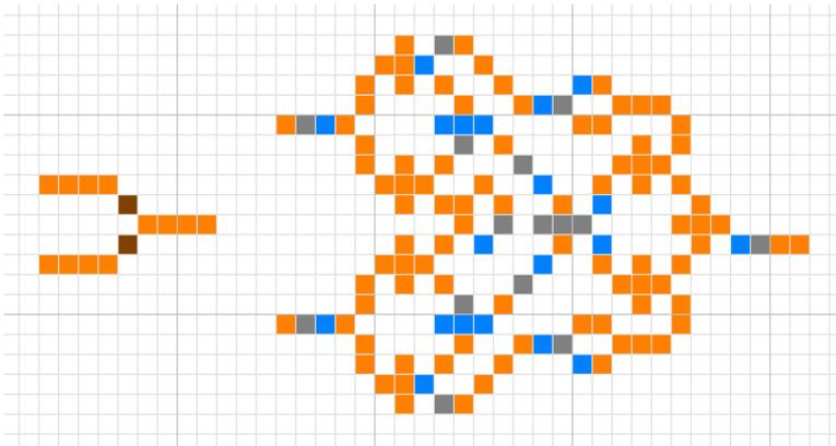
**Figure 17.** A Wireworld++ AND gate (left) and a Wireworld AND gate (right) for signals of period  $n \geq 3$ .
