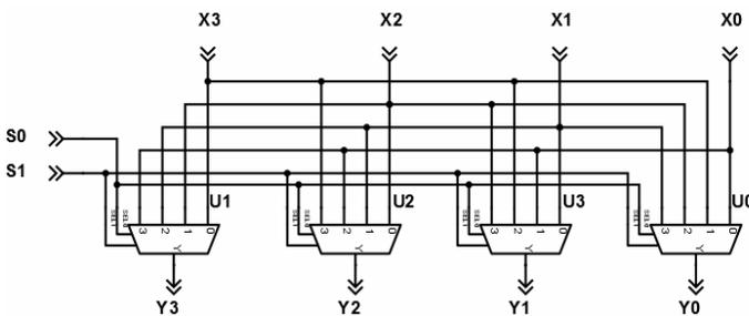
**Figure 2.** A 4-bit barrel shifter implemented using 4-to-1 multiplexers [12].
