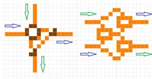
**Figure 13.** A Wireworld++ double-channel wire crossing (on the left), and an analogous Wireworld intersection (on the right) designed by Scherer. Both wire crossings are unidirectional and work correctly for signals of period  $n \geq 5$ . The arrows of different colors show the paths of each signal.
