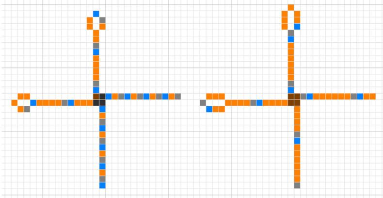
**Figure 10.** The signal 101010... travels along one wire, and the signal 010101... travels along the perpendicular wire. The signals in the configuration on the left have period  $n = 3$ . They cannot pass through the intersection correctly. The signals in the configuration on the right have period  $n = 4$ . The wire crossing works perfectly for them.
