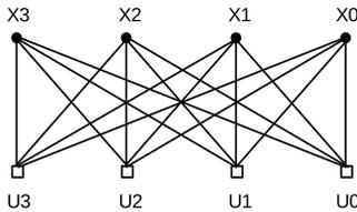
**Figure 3.** A graph that models the circuit from Figure 2. Components (multiplexers) are represented by squares. Metallic interconnections are represented by dots.
