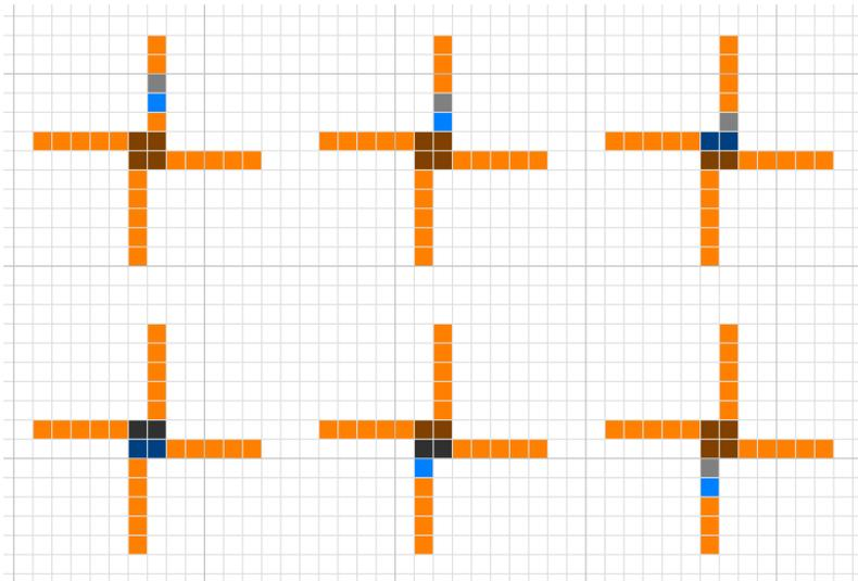
**Figure 8.** The successive snapshots of a single electron passing through the wire crossing (from left to right, top to bottom).
