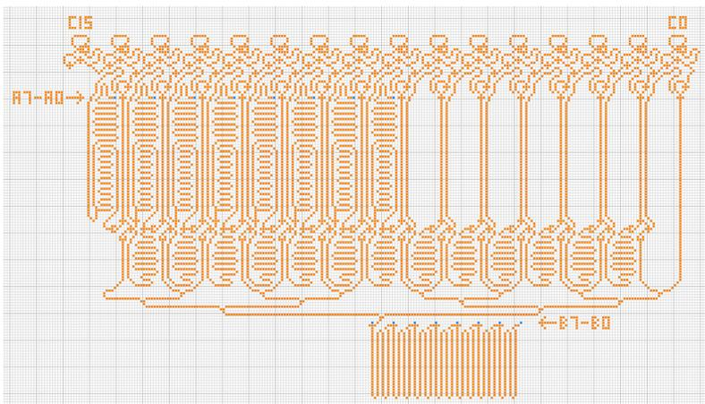
**Figure 1.** An 8-bit multiplier in Wireworld, designed by Gardner [8].
