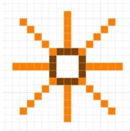
**Figure 12.** Four unconnected wires cross at one point. This wire crossing is single channel, bidirectional.
