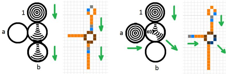
**Figure 21.** Similarities between implementations of a NOT gate in the BZ reaction [32] and in Wireworld++.
