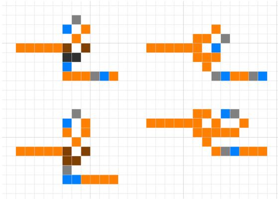
**Figure 19.** Wireworld++ NOT gates (left) and Wireworld NOT gates (right). The gates in the top row are for signals of period  $n = 4$ . The gates in the bottom row are for signals of period  $n = 6$ .
