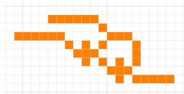
**Figure 18.** A Wireworld AND gate for signals of period  $n \geq 5$ .
