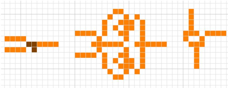
**Figure 20.** A Wireworld++ XOR gate for signals of period  $n \geq 3$  (left) and Wireworld XOR gates. The gate in the center works for  $n \geq 3$ , while the gate on the right works for  $n \geq 5$ .
