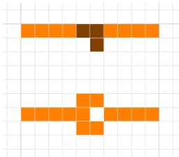
**Figure 16.** A Wireworld++ diode (top) and a Wireworld diode (bottom).
