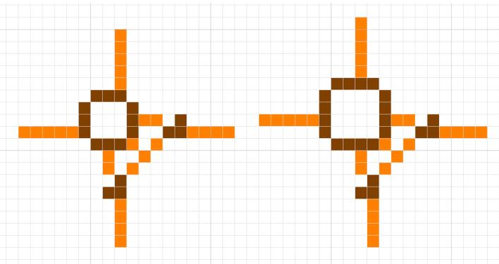
**Figure 14.** Double-channel wire crossings that work for signals whose period is not less than a specified number  $n$ . The smallest period  $n$  is uniquely determined by the perimeter of the central arrangements of weak cells.
