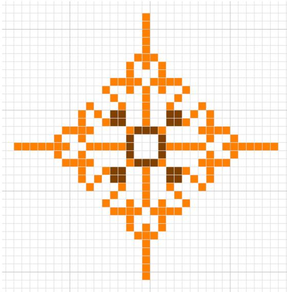
**Figure 15.** A double-channel, bidirectional wire crossing for signals of period  $n \geq 6$ .
