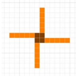
**Figure 7.** A bidirectional, single-channel wire crossing for signals of period  $n \geq 4$ .
