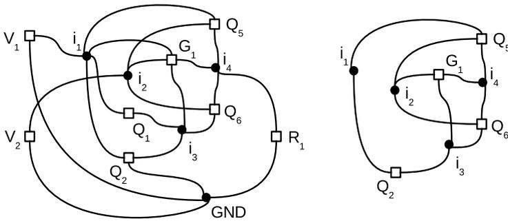
**Figure 5.** A graph that models: (a) the XOR gate from Figure 4; and (b) its subgraph that is a subdivision of  $K_{3,3}$ .
