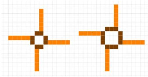
**Figure 11.** Wire crossings that work only for signals whose period is not less than a specified number  $n$ . On the left is a wire crossing that works only for signals of period  $n \geq 5$ . On the right is a wire crossing that works only for the signals of period  $n \geq 6$ . The generalization for larger  $n$  is straightforward.
