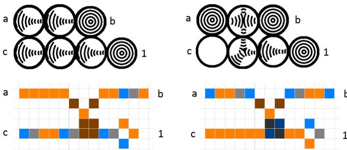
**Figure 22.** Similarities between implementations of a NAND gate in the BZ reaction [32] and in Wireworld++.
