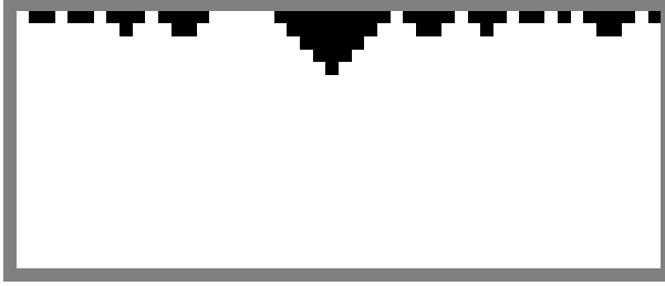
Figure 1. Example space-time diagram for ECA 128 (see section 2.2 for coding). Configurations are displayed horizontally and time goes from top to bottom.
