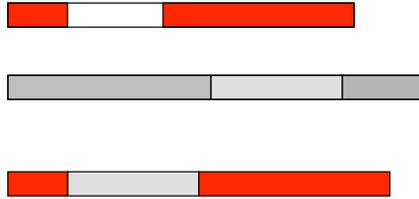
**Figure 2.** GPengine crossover. Two instructions are randomly chosen in each parent (top two genomes) as cut points. If the code to be inserted from the second parent at least partially overlaps the first, it is inserted in the normal way to give the child (lower chromosome). With headless chicken crossover, the inserted code is randomly generated.
